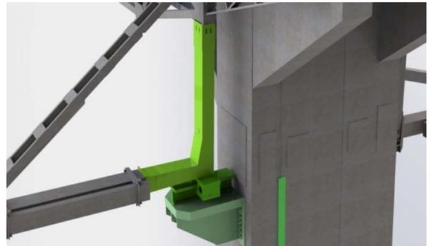
Figure 1. Illustration showing developed solution (highlighted) with part of deck truss replaced and supported by a new bearing on a new support bracket which projects out from the tower
