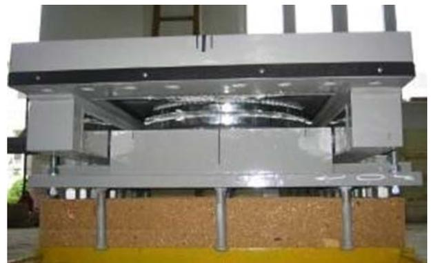
Figure 2. A guided sliding spherical bearing
